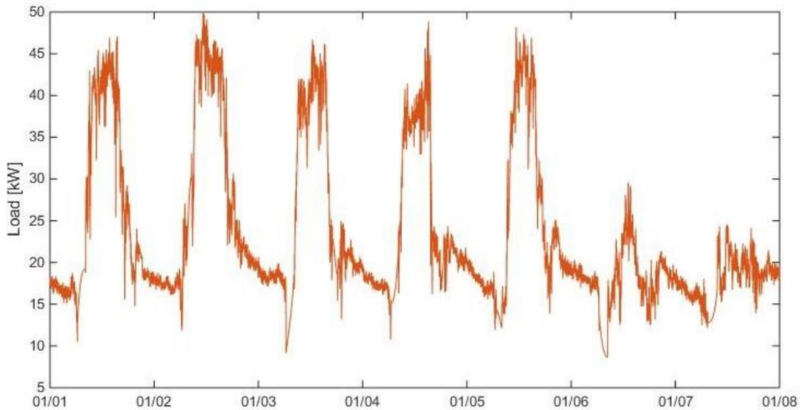
**Figure 8 – Average weekly load profile with complete load demand**
