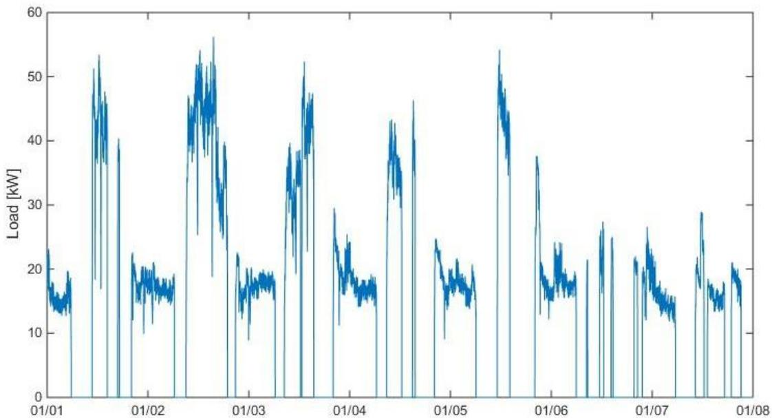
**Figure 7 - Weekly load profile example from current demand**
